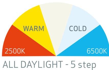
The new range reflects the entire colour temperature spectrum which occurs during the day and offers the option to choose between 5 different colour temperatures ranging from 2500K to 6500K.
